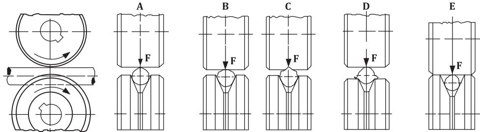
**Figure 9 : Pressure Setting and Roller Selection Mistakes**
