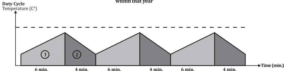
As defined in the standard EN 60974-1, the duty cycle rate includes a time period of 10 minutes. For example, if a machine specified as 250A at %60 is to be operated at 250A, the machine can weld / cut without interruption in the first 6 minutes of the 10 minutes period (zone 1). However, the following 4 minutes should be kept idle for the machine cool down (zone 2).
